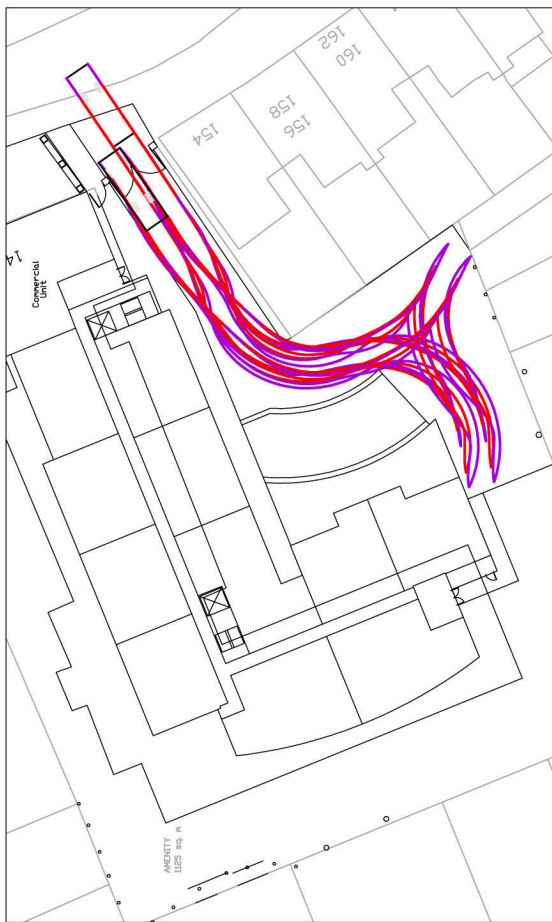
LARGE REFUSE MOVEMENT - IN & OUT
